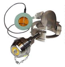
A Burst Disc Indicator is a simple circuit, usually fitted downstream of the bursting disc, which is broken on rupture. Marston manufacture burst indicators which are fitted directly to the disc as shown and to fit between the holder and the downstream pipe flange
